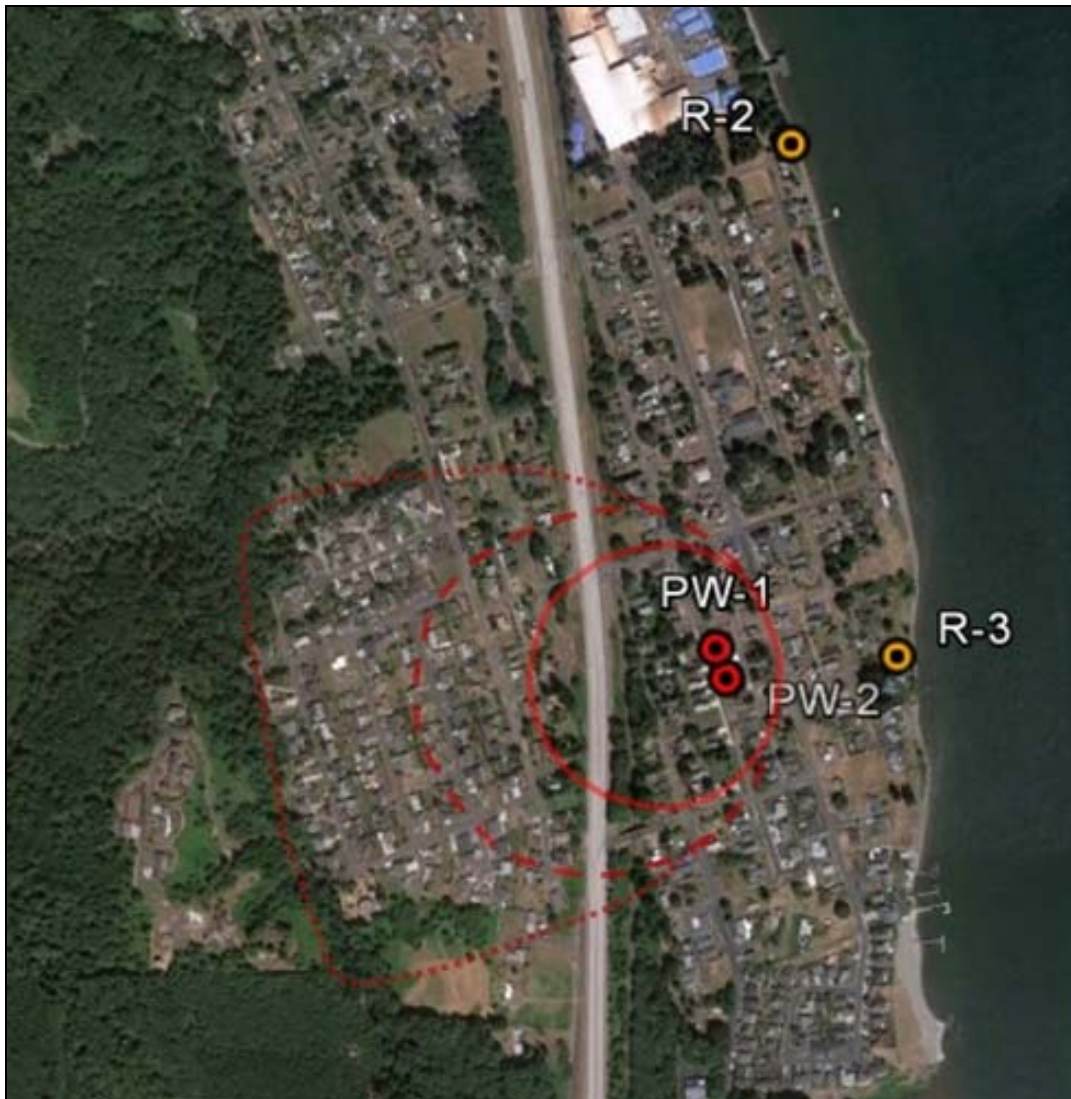
Figure 5 shows the delineated SWPA of the combined wells. The solid red line is the 1 year Time-of-Travel (TOT) zone, the dashed line is the 2 year TOT, and the dotted line is the 5 year TOT.
